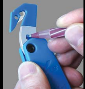
FILM CUTTER CHANGE Use ball point pen (above) to remove & replace film cutter unit.
