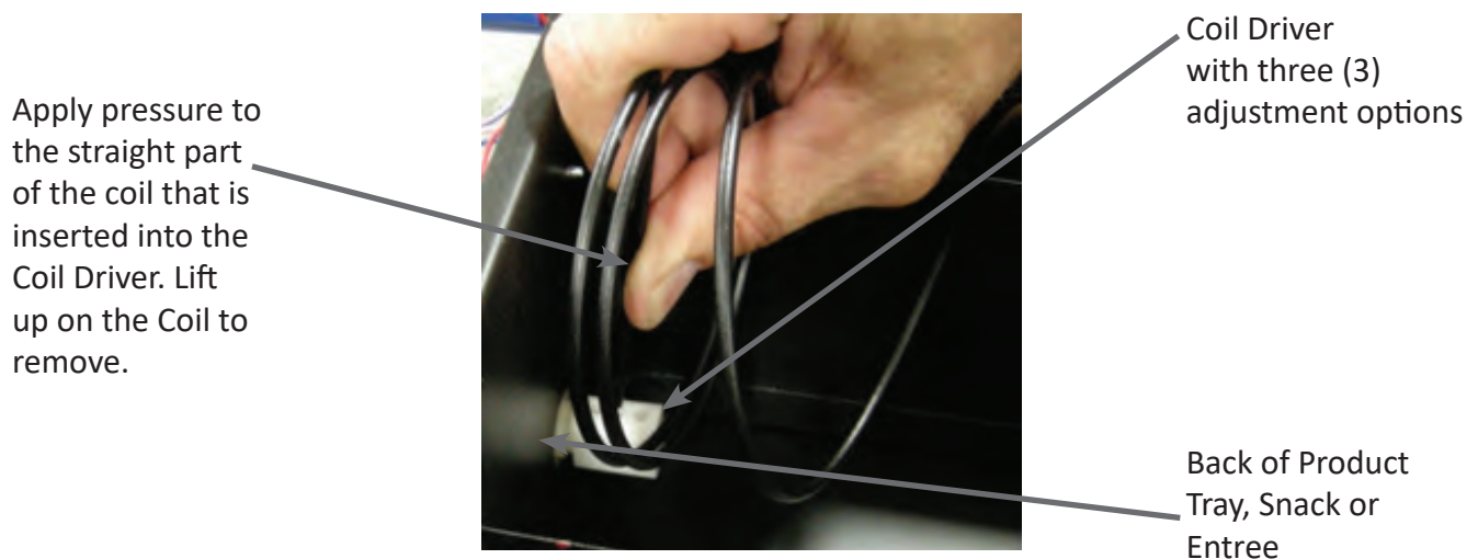
Figure 9 – Removing and Aligning a Coil
