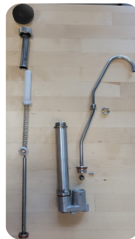
Pump Discharge Tube Unassembled & Plunger Fully Unassembled
