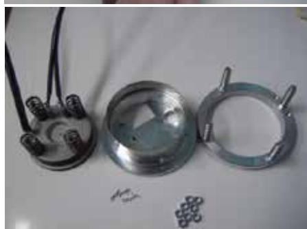
Graph 7-2 、 3 Using a wrench and box end wrench to separate the knife and heater. Then you can clean the mould and parts.
