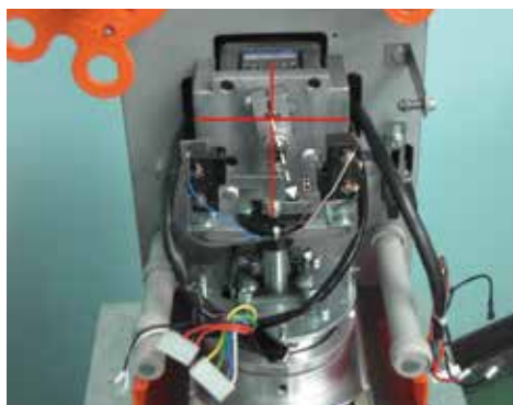
Graph 6-2 Move the lower micro switch to the right position-match.
