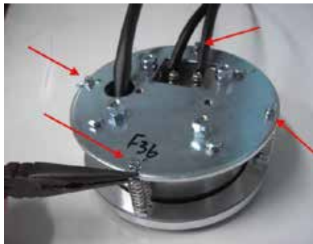
Graph 7-1 Using a clam strip down four B TYPE CLIPS, then take off the plate.
