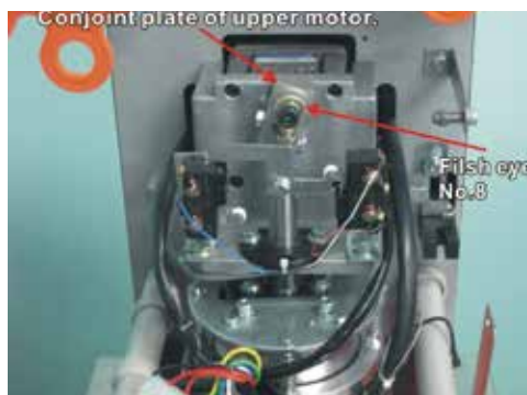
Graph 6-1 TO lubricate axle and fish eye No.8 once for a month.
