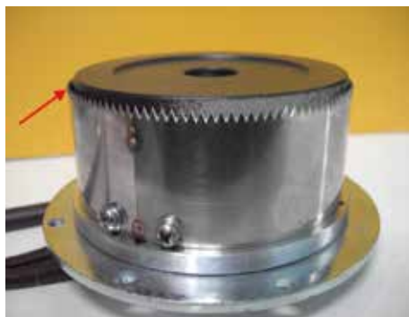
Graph 8-1 After cleaning, heater's position should be higher than the knife for 1mm.
