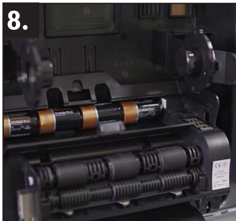
Load 4 D-cell Alkaline batteries as shown. Batteries must be loaded in the correct orientation, with positive end towards the left. If batteries are not loaded correctly, unit will not function.
