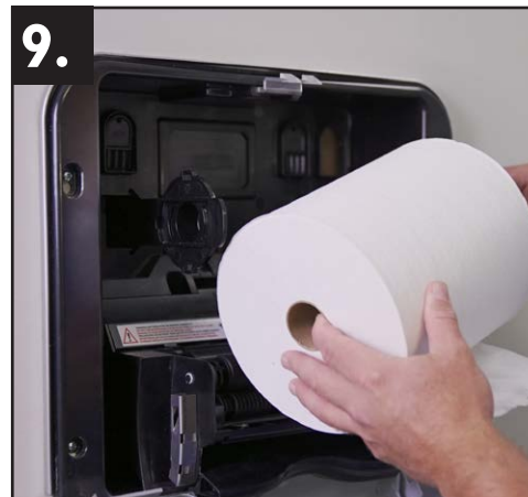
Load paper onto hubs. Pull down and drape so that paper is hanging off the back of the roll. Pinch paper by rolling between two rollers. Close cover. Dispenser will feed the first sheet and is ready to use.
