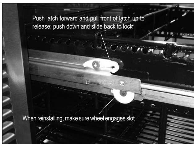
Figure 15. Removing/Installing Drawer
