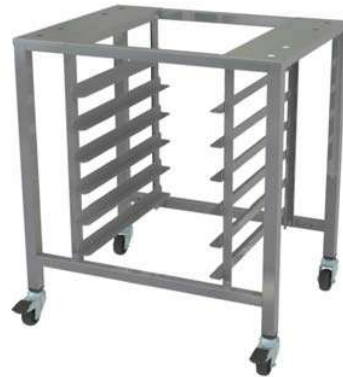
SK2731U - Stand for E27 / E28 810mm/32"(W) x 650mm/25 \frac{1}{2} "(D) x 900mm/35 \frac{1}{2} "(H) Accepts US \frac{1}{2} and US full pan
