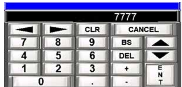
Fig. 76 - Keypad (Enter 7777 and ENT).
