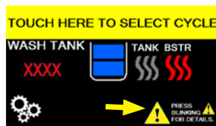
Fig. 102c - Main screen with blinking fault icon
