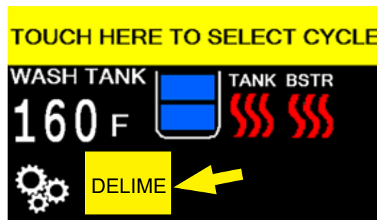
Fig. 80 - Main screen Delime button
