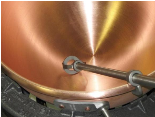
Temperature sensor probe for kettle
