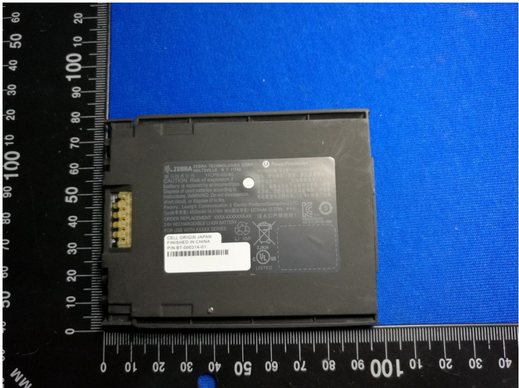
Battery (BT-000314-01 3,6V 4530mAh 16,31Wh(typ) 4270mAh 15,37Wh(min))
