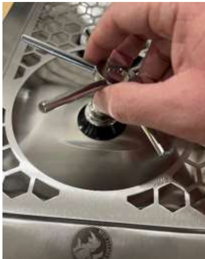
(A) Replace the actuator star over the valve body.
